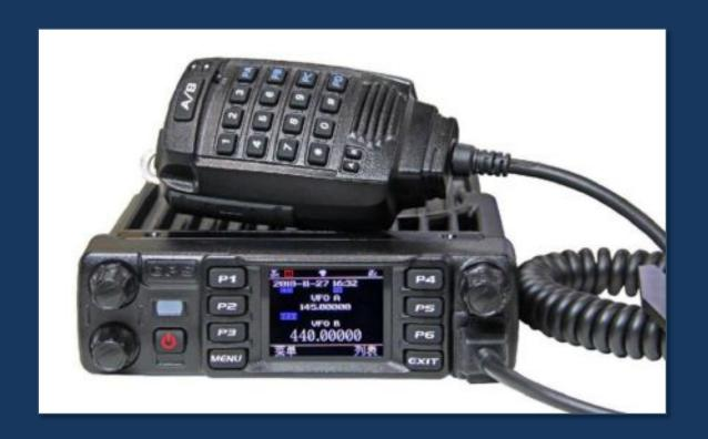
DMR/analog on all bands; first cross-mode rig (DMR to analog, analog to DMR)
